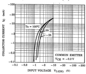
Fig. 10.4 RN2404 I<sub>C</sub>-V<sub>I(ON)</sub>
