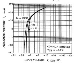
Fig. 10.5 RN2405 I<sub>C</sub>-V<sub>I(ON)</sub>
