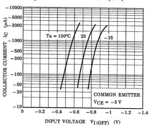
Fig. 10.12 RN2406 I<sub>C</sub>-V<sub>I(OFF)</sub>
