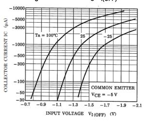
Fig. 10.10 RN2404 I<sub>C</sub>-V<sub>I(OFF)</sub>
