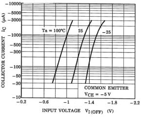
Fig. 10.8 RN2402 I<sub>C</sub>-V<sub>I(OFF)</sub>
