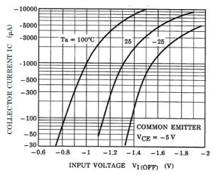
Fig. 10.9 RN2403 I<sub>C</sub>-V<sub>I(OFF)</sub>
