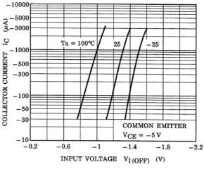
Fig. 10.7 RN2401 I<sub>C</sub>-V<sub>I(OFF)</sub>
