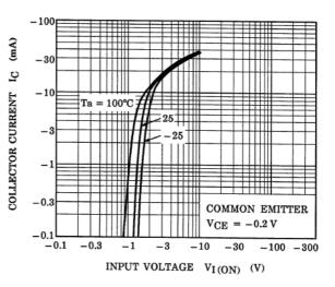
Fig. 10.2 RN2402 I<sub>C</sub>-V<sub>I(ON)</sub>
